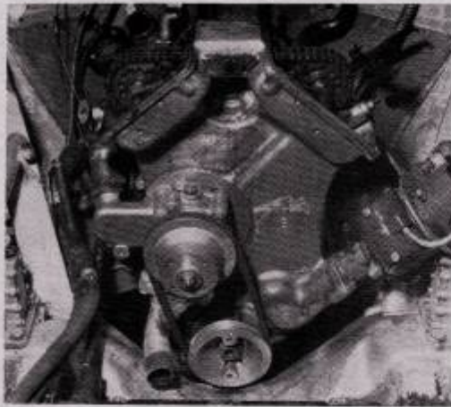
Cam drive is two-stage, by gear and chain. Large-capacity water pump has engine-speed belt drive, and special ignition angles to right.
